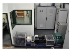
The university researchers had a demanding list of specifications, including regeneration capability and flexibility. So any supplier had to provide matching motors and drives, custom options (two shafts and a through-hole resolver, for instance) and a wound-rotor induction machine – unusual at this power level.
